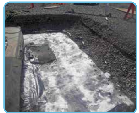
The surface of the contaminated Alabsorb layer had noticeable gelling, which indicated a reaction with oil.
