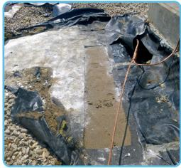
Albasorb was spread on the sand layer (left). A strip of **Oilmat** was placed overlapping the existing Oilmat, and more Albasorb was spread on top and around the seams of the new Oilmat strip (right).
